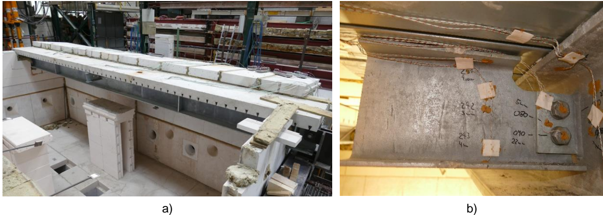
Figure 2: Large-scale fire test setup: furnace and composite beams (a) and temperature measurement at connection detail (b) (TU Braunschweig)
