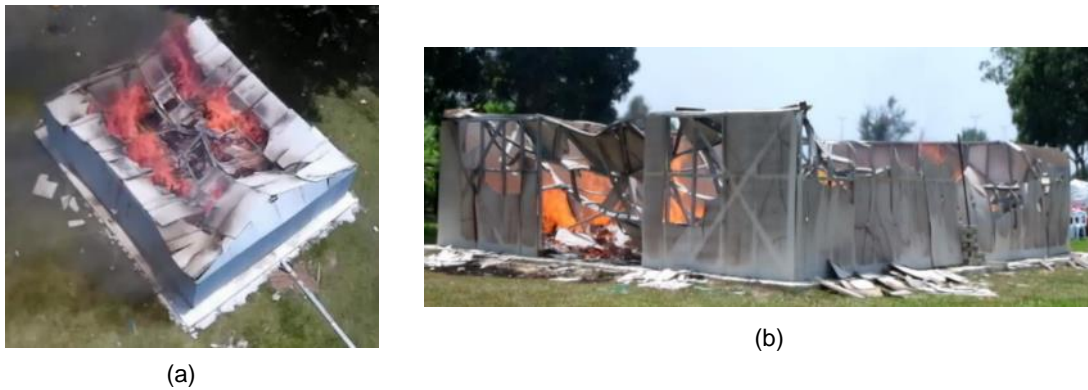
Figure 17 Structure during experiment (a) non-symmetrical collapse (b) Inward structural collapse (t = 38 min) [19]
