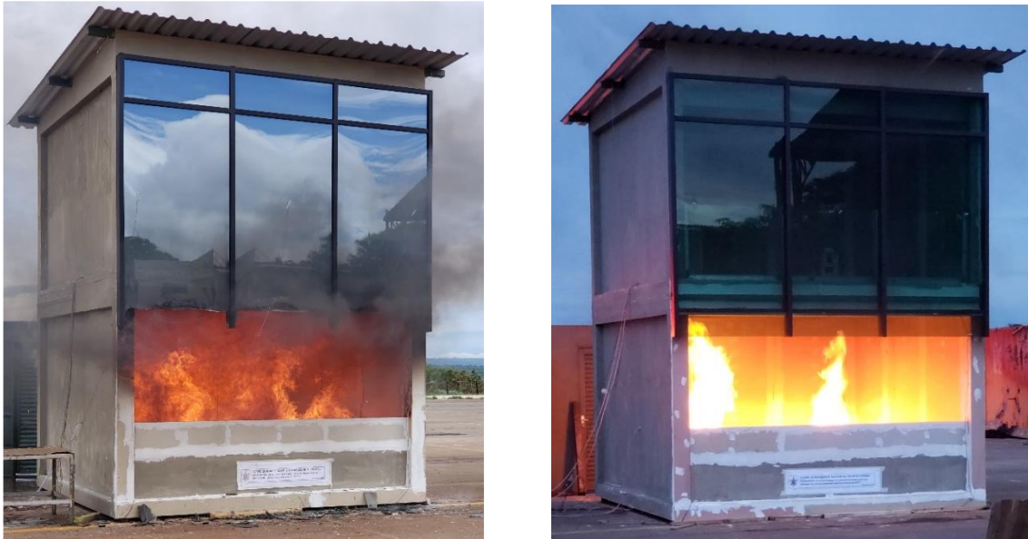
a) Experiment 1 - flashover phase of fire. b) Experiment 2 – The initial phase of fire Figure 5: Full-scale experiments of fire. (author)
