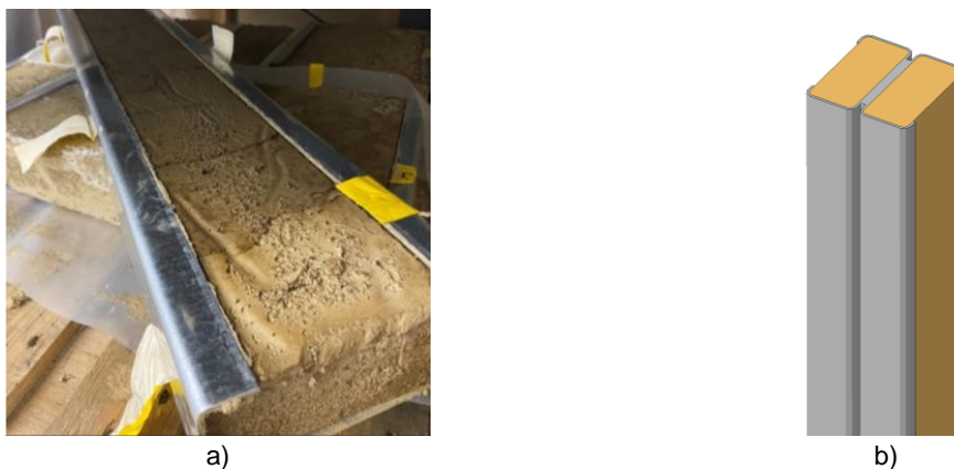
Figure 1: Production of “Stahlkammer” specimen and concept of a “Stahlkammer” column
