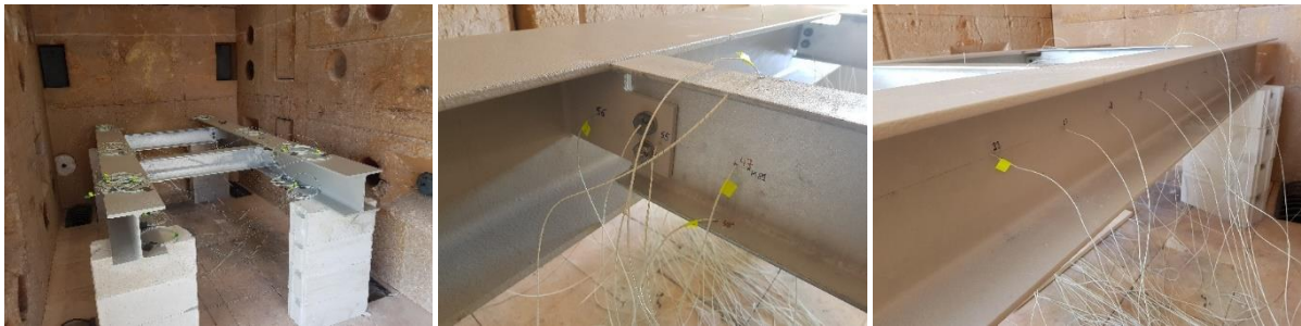
Figure3: Experimental setup unloaded beam tests (TU Munich)
