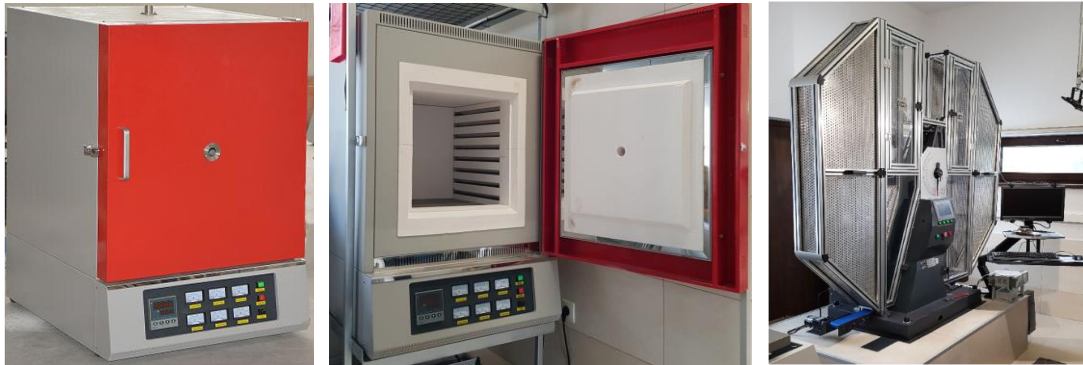
Figure 2: Equipment used to conduct the tests: muffle furnace KJ-M1200-64L-IC (at left and in the center), instrumented Charpy hammer JB-W450E-L (at right).
