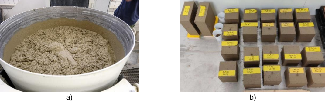
Figure 4: Mixing and curing of Cleancrete specimens in the climate chamber.
