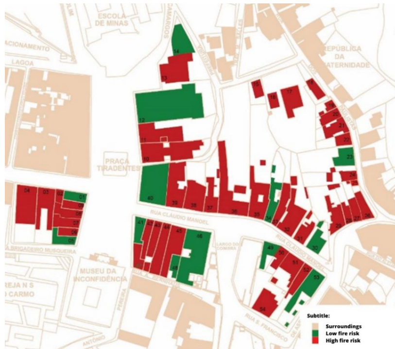
Figure 4: Buildings with low risk of fire and with very high or imminent risk according to the Simple Arica methodology (Pereira, 2022).
