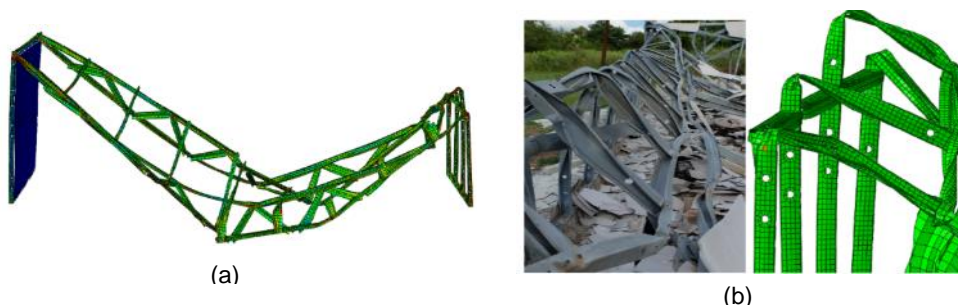
Figure 19 (a) Structure deformation obtained by numerical analysis (b) Experimental and numerical structural deformation comparison [19]
