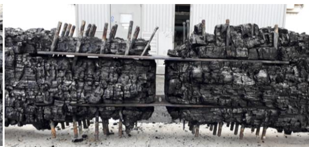
Figure 12: Failure mode of connection n°7'
